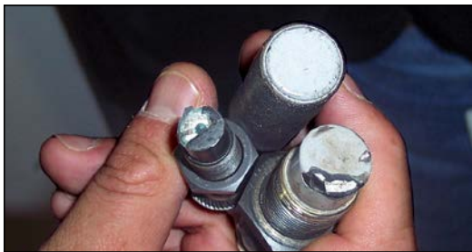
These sensors have been destroyed by impact or abrasion. One-piece stainless steel sensors are the go-to sensors for harsh sensing environments. They can take brutal punishment and still keep functioning.
