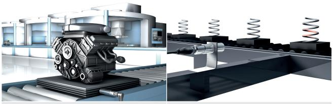
Inductive sensors detect workpiece carriers at close range simply and cost-effectively.
