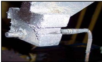
Unprotected sensor/cable connections can cause expensive unplanned downtime.
