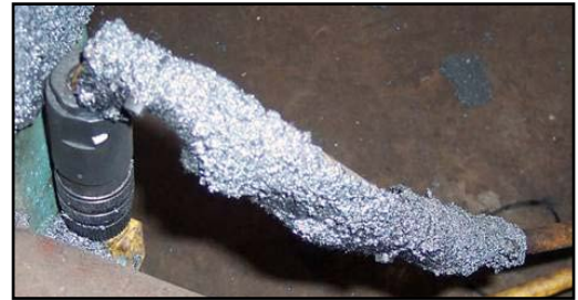
Slag built up slowly on this cable until the weight pulled the connection apart.
