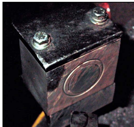
Prox sensor correctly protected against impact
