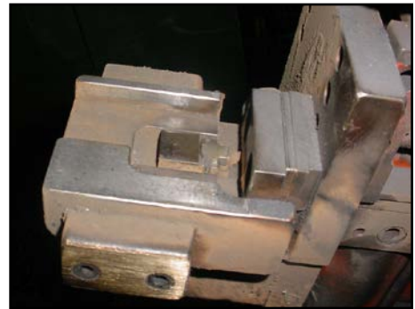
This sensor has a slag resistant coating that dramatically increases its life.
