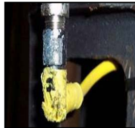
Unprotected sensor/cable connections can cause expensive unplanned downtime.
