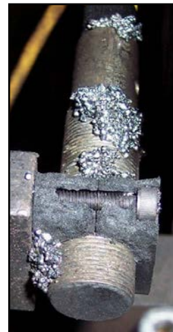
Prox sensor correctly protected against impact
