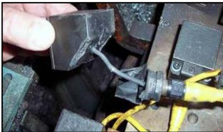
Loading impact can destroy unprotected sensors
