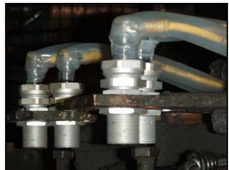
Now that these sensors and their connectivity are correctly protected, they should last for months—not just days.
