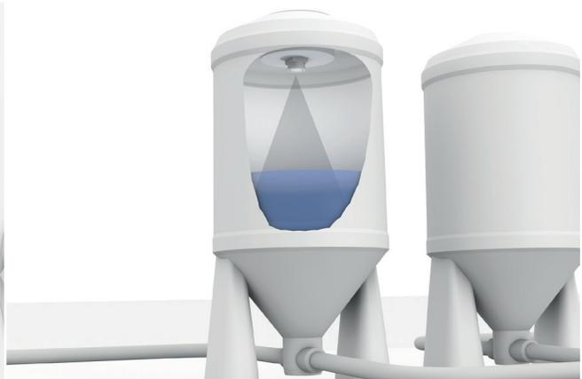
Level measurement of liquids in a tank using ultrasonic sensors
